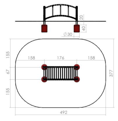
The equipment should be mounted on the ground in accordance with the Construction Declaration of the product through concrete foundations with the required dimensions or through anchoring to the existing concrete slab with a thickness at least 10 cm, which is reinforced in the anchoring area.
