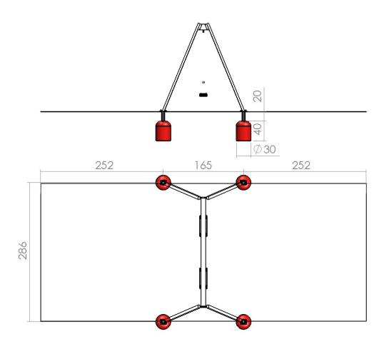
The equipment should be mounted on the ground in accordance with the Construction Declaration of the product through concrete foundations with the required dimensions or through anchoring to the existing concrete slab with a thickness at least 10 cm, which is reinforced in the anchoring area.
