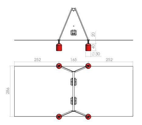
The equipment should be mounted on the ground in accordance with the Construction Declaration of the product through concrete foundations with the required dimensions or through anchoring to the existing concrete slab with a thickness at least 10 cm, which is reinforced in the anchoring area.
