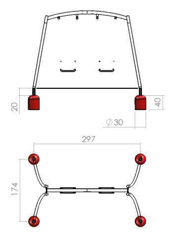
The equipment should be mounted on the ground in accordance with the Construction Declaration of the product through concrete foundations with the required dimensions or through anchoring to the existing concrete slab with a thickness at least 10 cm, which is reinforced in the anchoring area.
