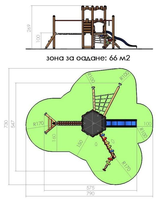
2. Dimensions of the Equipment and Minimum Space for Placement
